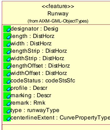
Figure 4: Runway class showing the newly added centerlineExtent geometry reference
