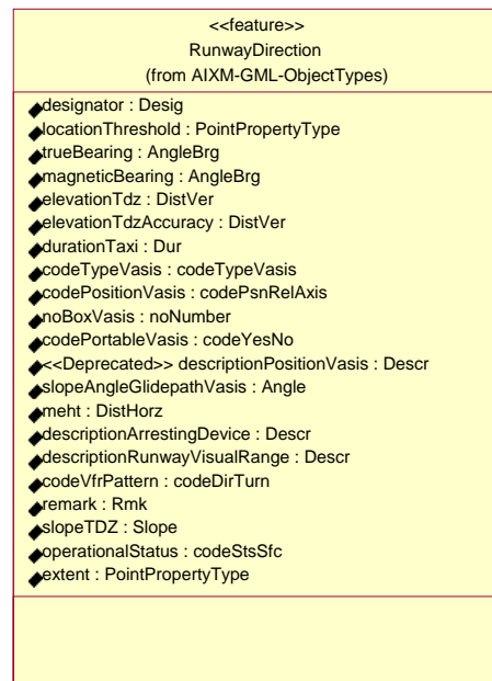
Figure 2: RunwayDirection class showing the newly added slopeTDZ attribute
